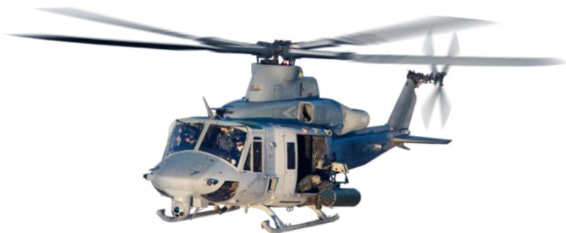
Combat-proven utility helicopter supporting U.S. Marine Corps global missions over the next 40 years. Integrated avionics and glass cockpit. Fully marinated against harsh desert and maritime environments. 85 percent of parts common with the AH-1Z.
